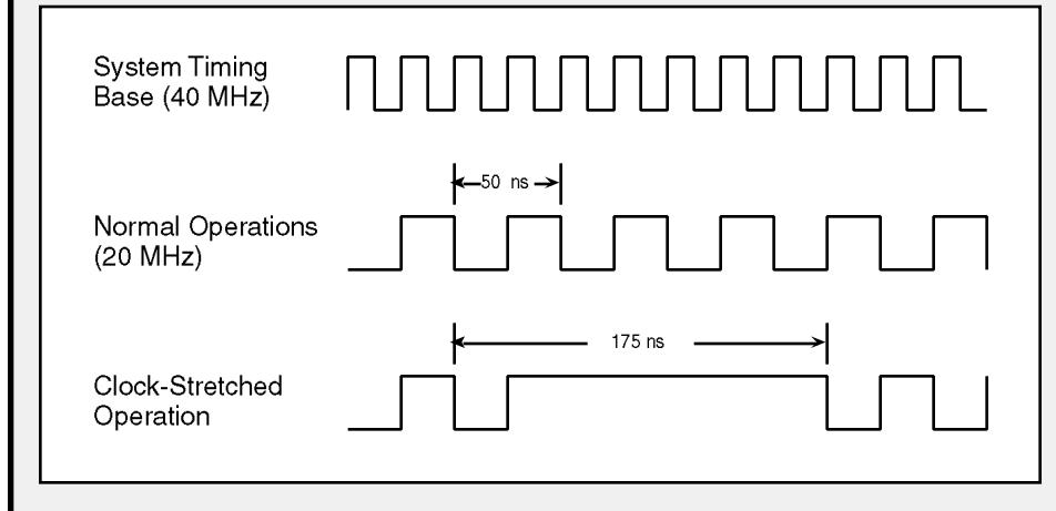
approximately every 10 microseconds (about 200 cycles) and can cause a 1 cycle DRAM memory operation to take up to 8.5 cycles to complete. We could see up to 11 refreshes while executing a 2 KB segment of code, so if take this into consideration, our throughput drops to about 19.2 MHz.
