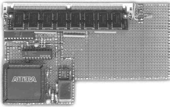
memory mapping, control and refresh circuitry. While this vastly decreases the amount of board space required, developing the logic equations needed to program the chip for a specific function often proves to be very time-consuming.
